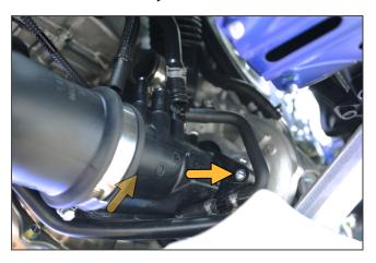
4) Install the Hybrid valve, then reconnect the vacuum hose, the two hoses in front of the valve, and the turbo intake pipe, making sure to replace and tighten all bolts and hose clamps.
