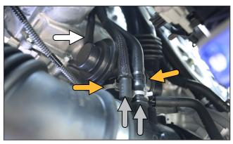
3) Using a 10mm socket, remove the two bolts that hold the turbo intake pipe onto the turbo.
